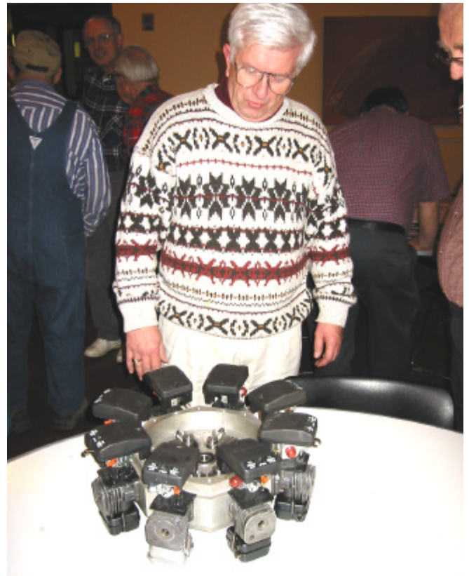
8 Cylinder Radial Weed-Wacker Photo by John Wasser
