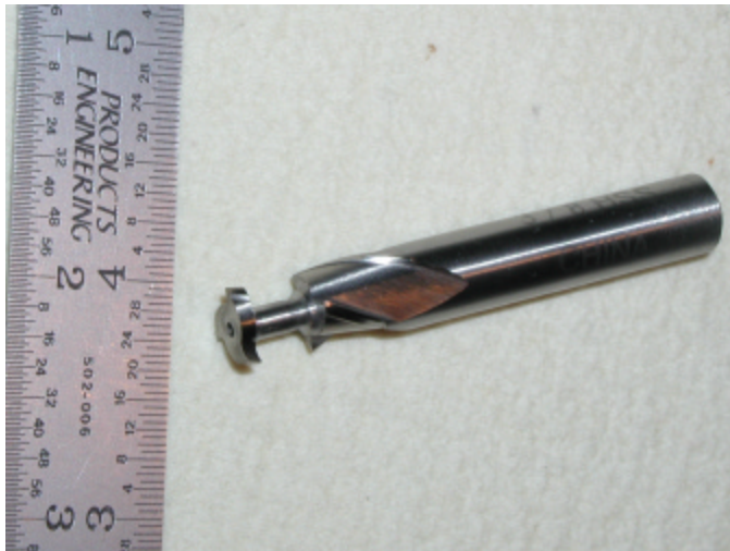
Shop Made Tee Slot Cutter
