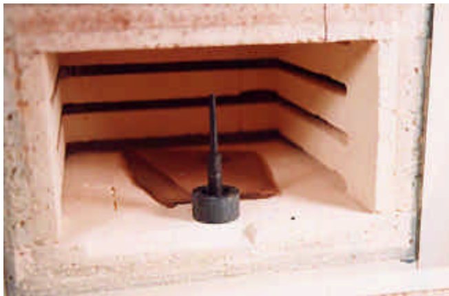
A2 reamer blank held vertical in oven to avoid sagging Photo by Larry Twaits
