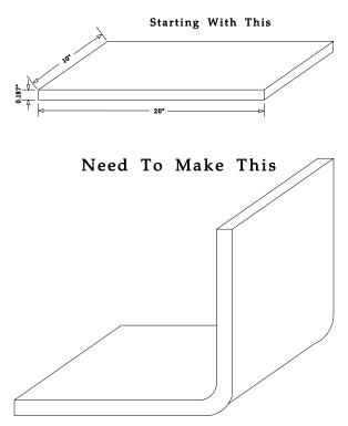
I asked for advice on the metalworking newsgroup and was told that I'd need 8 to 10 tons of force to bend that plate. Gosh, that rules out hand bending...or does it?
