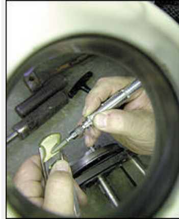
A magnifying glass aids in polishing the brass handle of a pocket knife.
