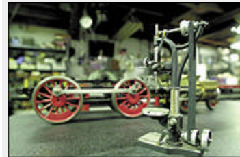
A model 1840s drill press built by Dick Boucher at a scale of one inch to one foot stands near a miniature train chassis he's restoring.
