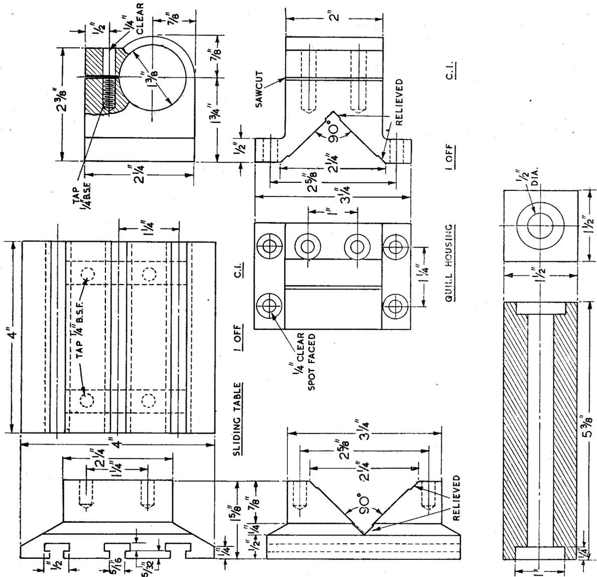
GENERAL ARRANGEMENT OF MILLING FIXTURE
