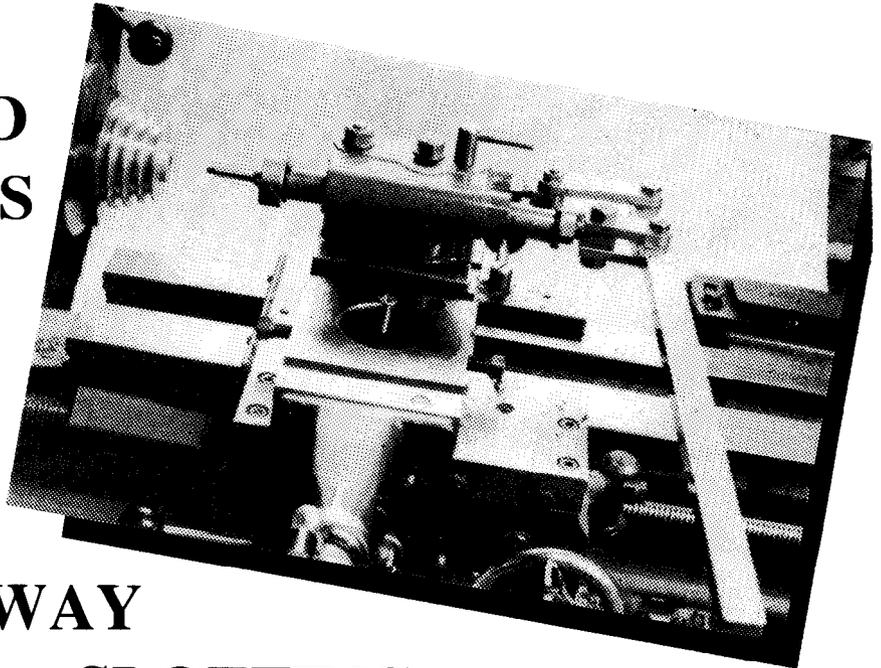
**CUTTING INTERNAL KEYWAYS** in the home workshop is an operation for which no specific equipment has been available for a long time, and never on a low-cost basis.
