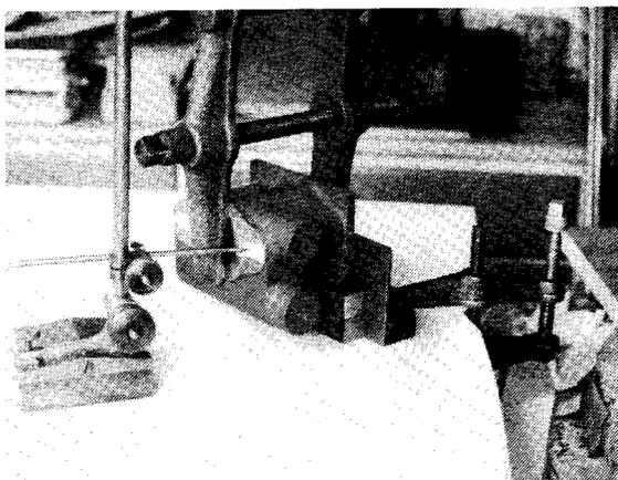
about the same size as the larger boss. Mark the centre of the hole for the ram, 1/2 in. in from the front of the casting, and cross wind the table to pick up this centre with a vee-pointed D-bit or a very short drill well nicked to thin the web at the end.
