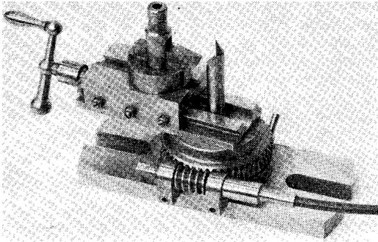
*Fig. 11. A worm-gear spherical turning appliance.*
