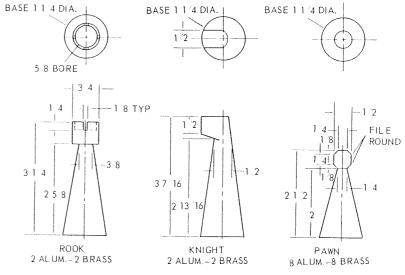
CHESS PIECES ARE TURNED FROM BRASS AND ALUMINUM BAR STOCK. IRREGULAR TOP SECTIONS MAY BE SHAPED WITH A BAND SAW, FILE AND BELT SANDER.
