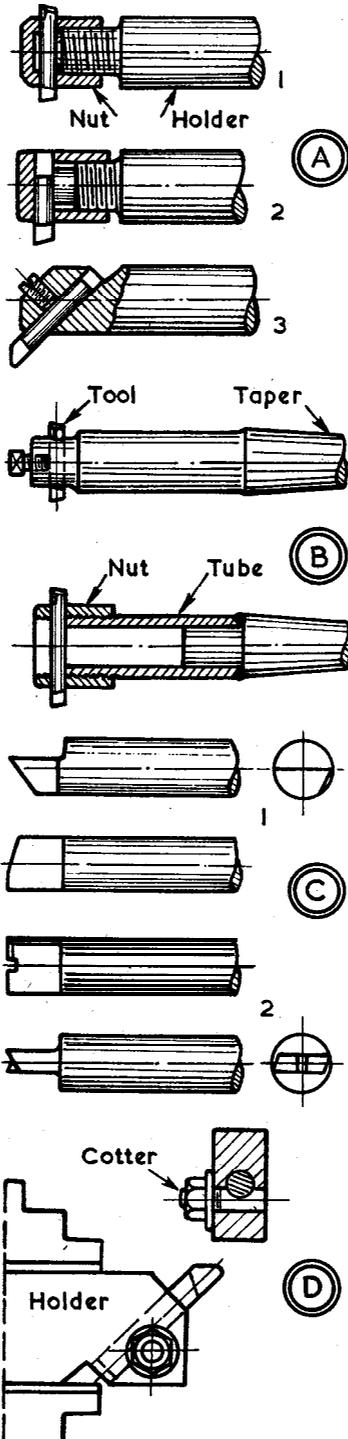
Holder 3 can be used in the two ways mentioned-in the chuck or on the topline, the angle mounting of the tool bit allowing it to work to shoulders or end-faces. To help in drilling the hole for the bit, a small flat can be filed on the holder where the drill is to enter, and another where it will emerge. This dodge helps reaming as well.
