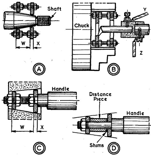
with the bore of one of the washers, the bulb lights up. By noting the light, or lack of it, as the tool is moved in the washers, you know how to set the slide. To make a check of concentric spinning, turn the chuck with the tool inside one of the washers.
