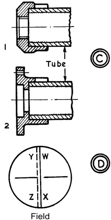
3/32 in. thick. Using the independent chuck, I turned S 3/4 in., T 1 9/32 in., U 1 3/16 in. to 1/16 in. deep. I made V 1/32 in. by filing and then case-hardened the end. The securing ring screwed out easily, bringing the field lens with it.
