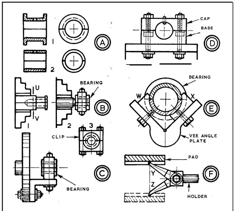
in a chuck, as at B2, with a clip B3 round the outside. Make this clip by boring two pieces of flat material in the independent chuck, after bolting them together.
