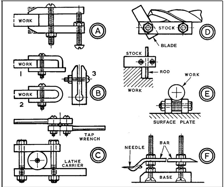
preference in lathe carriers is for the type illustrated. Both these tools can be made from square mild steel bar, even by novices. You should clamp the pieces for drilling to keep the holes in line. File matching Vs in the pieces for the tap wrench to locate and grip the tap by two corners of its square. Use a round file to produce shallow radii for work held in the carrier. You can turn each of the handles of the tap wrench in a lathe by holding one end
