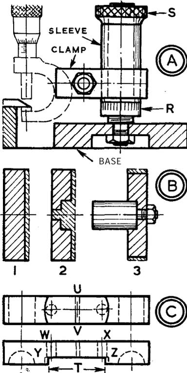
measure them in the normal way. When you need 2 in. with the spindle right up, you use a 1 in. block with a flat pointer on top to set the anvil, as shown. If you want 3 in., you build up 2 in. with a pair of 1 in. blocks.
