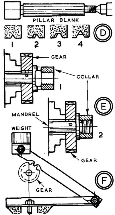
leaves them with half-circles **YZ**. Finally, each piece is held in the chuck to skim its inside face for clearance.
