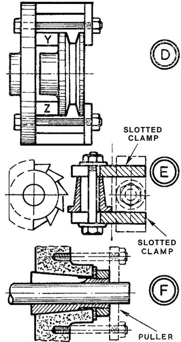
on the lathe faceplate. For boring the rear side, packing was placed to the faceplate, Y-Z. For boring the boss side, the pulley was clamped direct to the faceplate. With the use of topslide feed, the tapers were opened out until the dummy entered to a scribed line.
