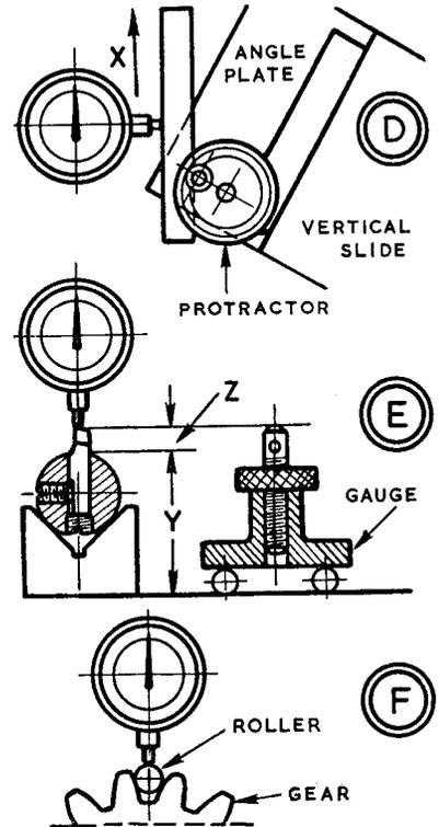
and for tapping the face of work, use a lead or hide hammer. If a faceplate wobbles, pack at the low point with paper. To true a button C, tap the edge of work with a brass or aluminium punch—the clamps can set a vertical slide to any angle just gripping. Then tighten them firmly.
