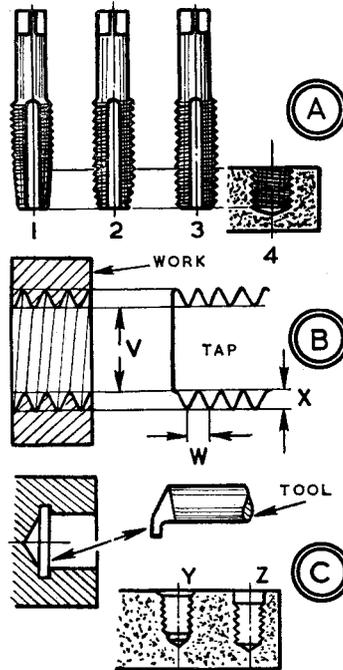
the core diameter (tapping drill size)  $V$  is obtained.
