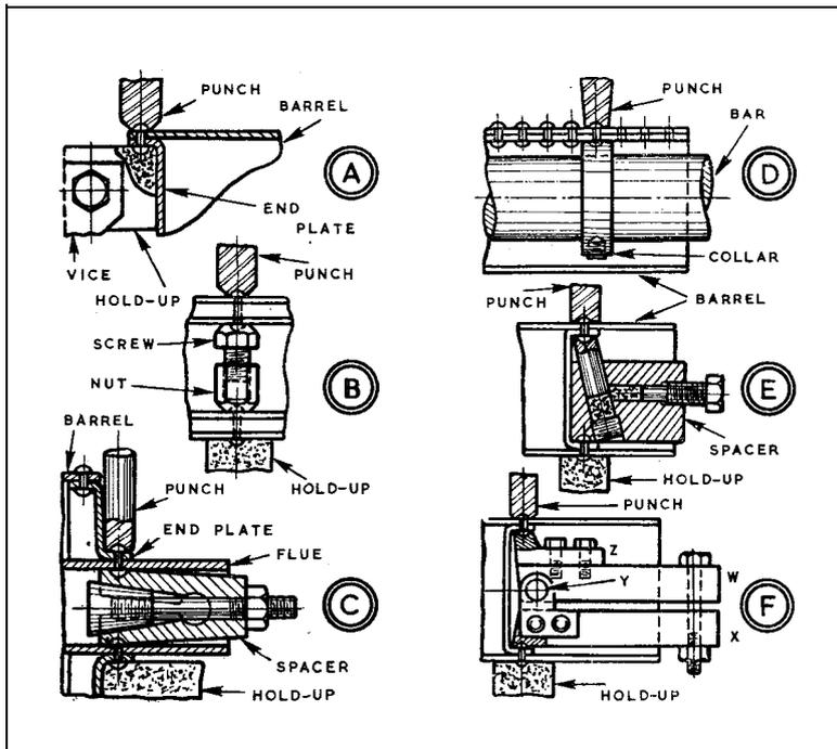
and punch can be used as at **A** with the hold-up gripped in the vice. Ordinary care gives a good result; and for a simple job, the endplate can be invisibly soft-soldered by fluxing in the barrel, putting in a lump of solder and heating, so that with tilting and turning the solder runs all round the joint. Tinning before riveting is helpful in this work.
