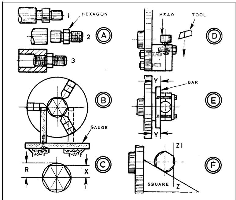
a gauge, **B**, and the three-jaw chuck. The two pieces of flat material are joined by countersunk screws, one bridging the bed, the other standing vertically to centre height. The vertical piece is faced in the independent chuck; and with an off-set, a step is turned to a depth of half the thickness of the jaws of the three-jaw chuck. One jaw is brought down to the step for setting, and the gauge is used each side of the blank with a hand scriber.
