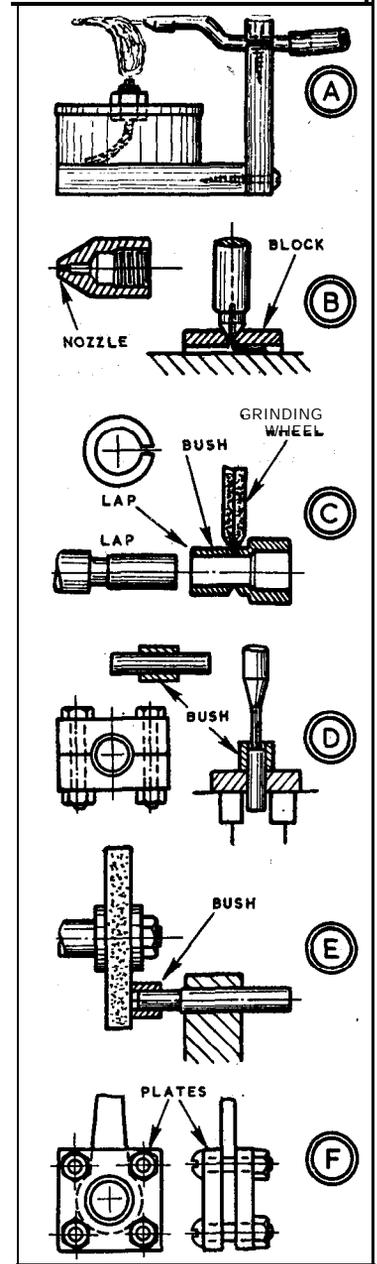
Clamping between thick steel plates, as at F is a way of reducing distortion in quenching on the boss of a rod whose bore is to be hardened. If it is casehardened, the compound is only put into the bore, so the outside of the rod remains soft. □
