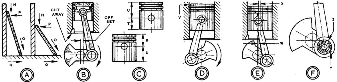
for dispersing heat and reducing weight, the considerable clearance which must be allowed for expansion can result in slap at TDC. It occurs when combustion pressure is applied, and may be aggravated or alleviated according to general proportions and layout.
