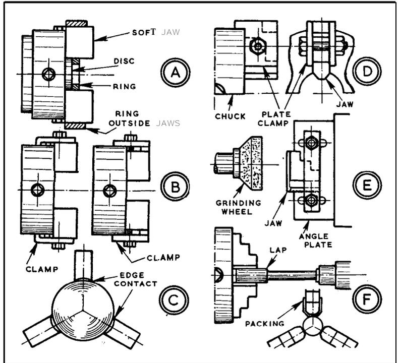
to fit clamps, as at B. For securing jaws inside the chuck diameter (right), each clamp can be straight and balanced by a small packing block. For securing, however, where jaws stand proud of the chuck diameter, each must be bent down (left). In both cases regulation of individual holding screws is necessary.
