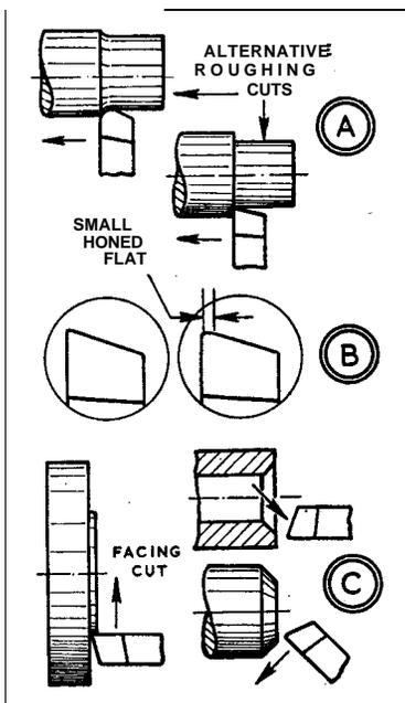
because of its longer cutting edge for a given depth of cut. On the other hand, a sharp round-nosed tool may not cause chatter where a blunt one would; and in a borderline case, the use of oil or cutting suds may prevent chatter-as against dry cutting.
