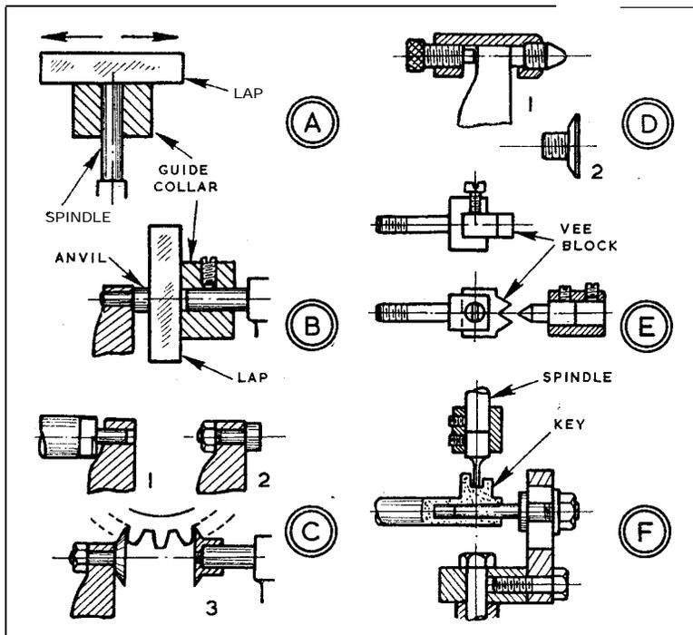
They should not be applied to running work, nor to dirty or abrasive surfaces—apart from the incorrect measurement which would result; and before the micrometer is finally closed to put away, a piece of clean notepaper should be lightly gripped between spindle and anvil, and drawn out from between them, thus taking any fine particles of dirt or abrasive with it.
