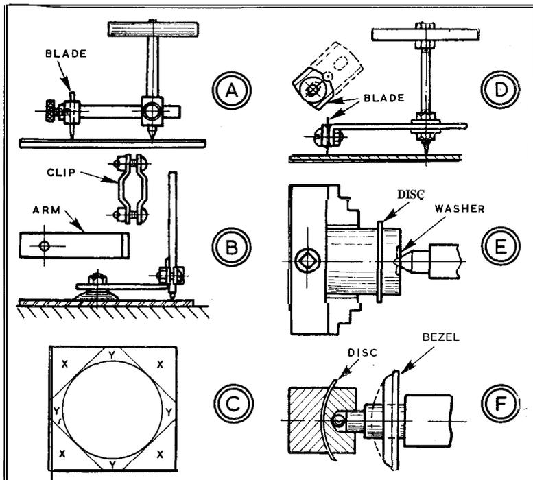
For materials like cardboard, fibre, composition sheeting, thin plywood, and even soft metal, the type of washer cutter at A is very suitable. With the blade set to radius and the centre point pressed well down, the tool can be turned in regulated cuts. Except on thin material which can
