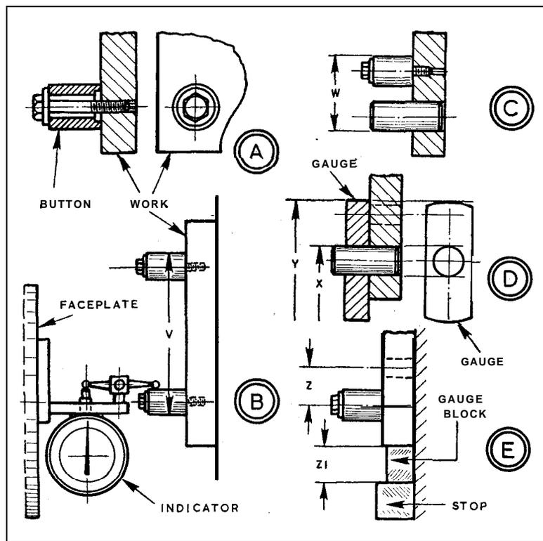
boring principle can be continued even to the locating of holes. That is, having settled the position of one hole by any method, the positions of others-can be obtained by appropriate feeds on the screws-afterwards clamping the vertical slide and cross slide.
