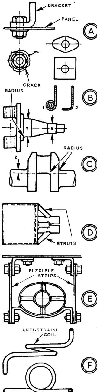
strain and vibration can be very prone to cracking; and unless there is some support for a panel at a bracket, a crack may completely encircle a bolt, as at A. In these circumstances large washers can effectively distribute strain over a wide area. They may be round, oval or square.
