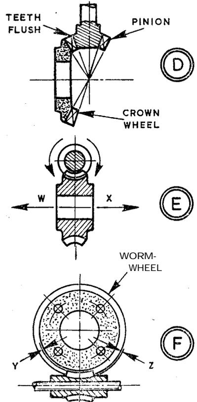
anti-clockwise rotation causes thrust in direction X. Incorrect centring or too much play can cause binding in one direction.
