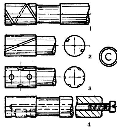
set up can be lapped holding the lap by hand, especially where such part may be a bush difficult to hold otherwise. The lap may then be somewhat shorter than when it is itself run in the lathe and the part applied to it.
