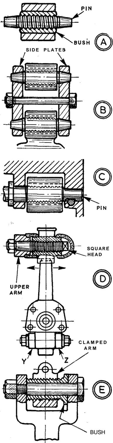
**A**LTHOUGH it is bad practice to employ screwed or threaded pins in plain holes where movement is to occur, yet properly designed assemblies of screwed pins and bushes can, where applicable, provide certain advantages by simplifying construction and furnishing means of particular types of adjustment.
