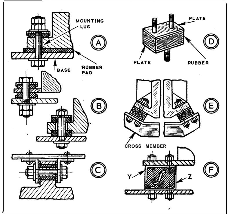
of vibration and noise absorption, from use of soft rubber padding below and rubber washers on top of mounting lugs—as at A. Advisedly, the holes in the lugs should clear the bolts—which should have flanged washers on the rubber washers to prevent splaying, plain washers, and lock-nuts for adjustment.
