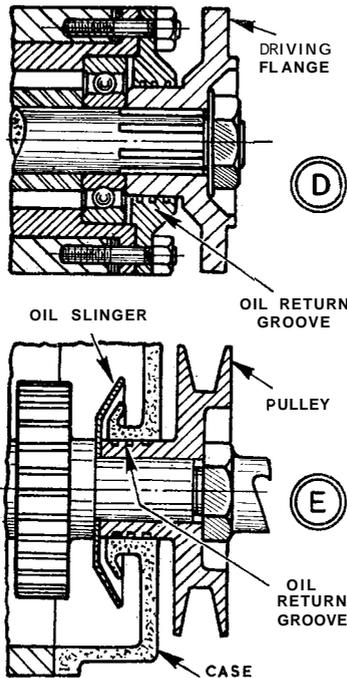
In the same way oil can be displaced between a shaft and bearing, or between a boss and the bore of an enclosing casing.
