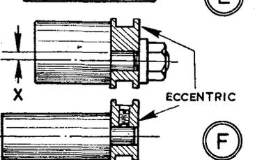
**M**OTIONS employing eccentrics are common in applied mechanics and can be arranged in several ways.
