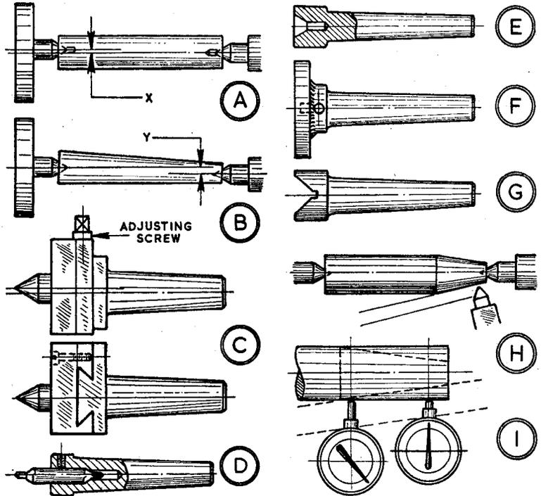
A centre drill for use from the tailstock can be mounted in a holder *D*. Mild steel is turned taper on the outside to fit in the lathe spindle, then centred with a pointed tool and drilled from the tailstock to take the centre drill tightly—a grub screw being used for holding. In the absence of other means of extraction flats can be filed on the holder to turn it with a spanner.
