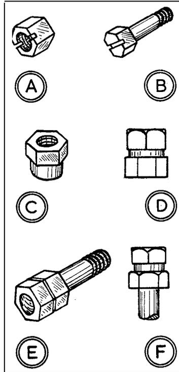
A deep bolt head, like a deep nut is often all that is required to facilitate assembly and dismantling. Special bolts can be turned from hexagon bar, a somewhat lengthy and deterring process, and another method, quicker and generally equally effective, is to braze an ordinary nut on top, E. If the double-hexagon principle is required as C can be used on the bolt somewhat shortened, F.
