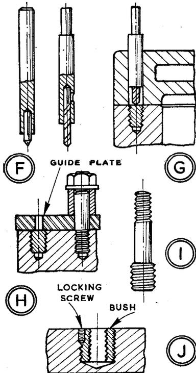
**I**N ASSEMBLIES where bolts would be impracticable, studs are an alternative to setscrews and, being permanently fitted, possess advantages.
