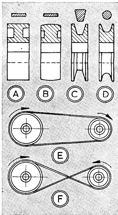
**O**F THE DIFFERENT means for transmitting power between shafts, belts and pulleys are undoubtedly the simplest and, within their application, possess virtues lacking in gears- and chain and sprocket drives.
