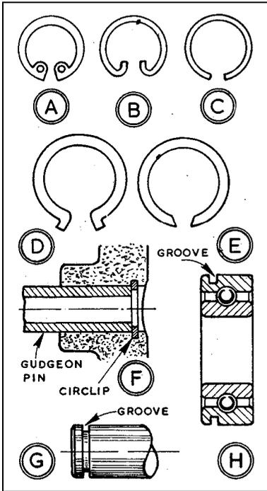
in half-round grooves may compress or expand (depending on the application) and push out. Such circlips should always be sunk in their grooves to at least half the diameter of their section. With circlips of soft material, which have to be squeezed into grooves, care must be taken to do this properly.
