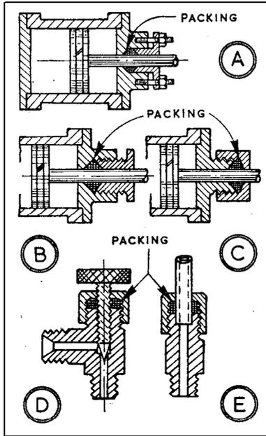
taps), and small needle valves, D. In the latter connection, it can be said that the packing will compress and seal in the thread, as shown, providing it is true and smooth, and an important saving in length can be made, by comparison with valves having a plain diameter for the packing to bear on.
