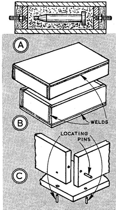
washers, and components on which distortion may be small or not important, can be case-hardened singly or in numbers by laying on a piece of sheet iron, heating to red, covering with compound, reheating, then quenching the lot. A shaft or spindle, however, on which distortion can occur, should be lifted off by pliers, plunged vertically and kept moving.
