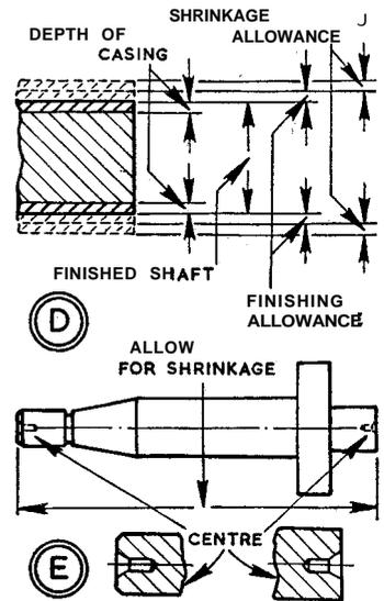
colour, and can be repolished with emery cloth-sufficient in most cases. On a shaft where size is important, however, allowance should be made of about 0.001 in. per inch of diameter for shrinkage, and 0.004 in. to 0.008 in. for finishing by grinding-the larger dimension also taking care of slight distortion. Several thou. depth of casing should then remain, D.
