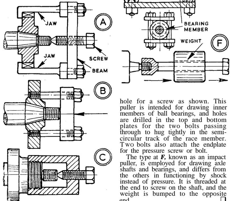
hole for a screw as shown. This puller is intended for drawing inner members of ball bearings, and holes are drilled in the top and bottom plates for the two bolts passing through to hug tightly in the semi-circular track of the race member. Two bolts also attach the endplate for the pressure screw or bolt.
