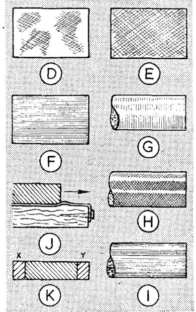
E-which is attractive when fine files are used. Uni-directional filing or draw-filing produces a finish as F, as is often done on tools.
