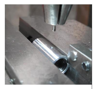
First note is how short the drill is being held. In normal life, we've been taught to never grip a drill by the flutes. But in this case, it avoids a center or spot drill operation, which would be needed if the drill was held "correctly". And using a split-point drill minimizes any wobble when starting the hole, as long as it's started gently. Of course the quill stop is set so that the chuck jaws don't hit the part.
