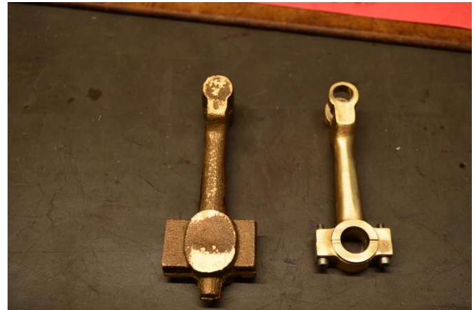
Photo 3 is from the May Gazette showing one connecting rod completed and the rough casting for the other. Photo 4
