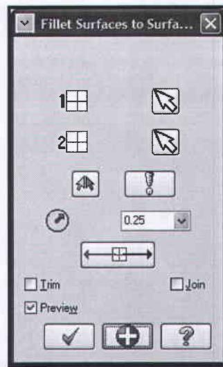
● The surface normals should always point toward the center curve of the resulting fillet surface.
