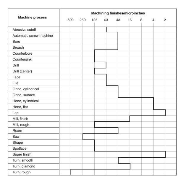
The finer the finish (the lower the roughness value in microinches), the higher the cost of obtaining it.
