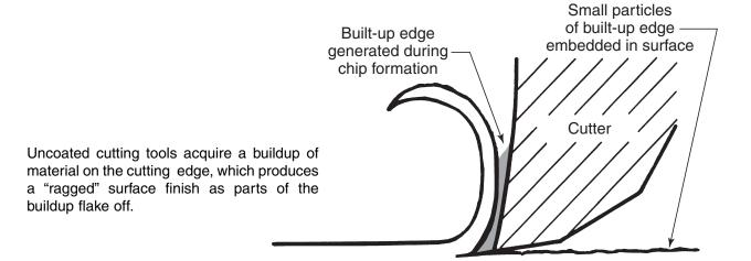
Tools coated with titanium nitride (TiN) and titanium carbide (TiC) resist the buildup from chips, run cooler, stay sharp longer, and produce a better surface finish.
