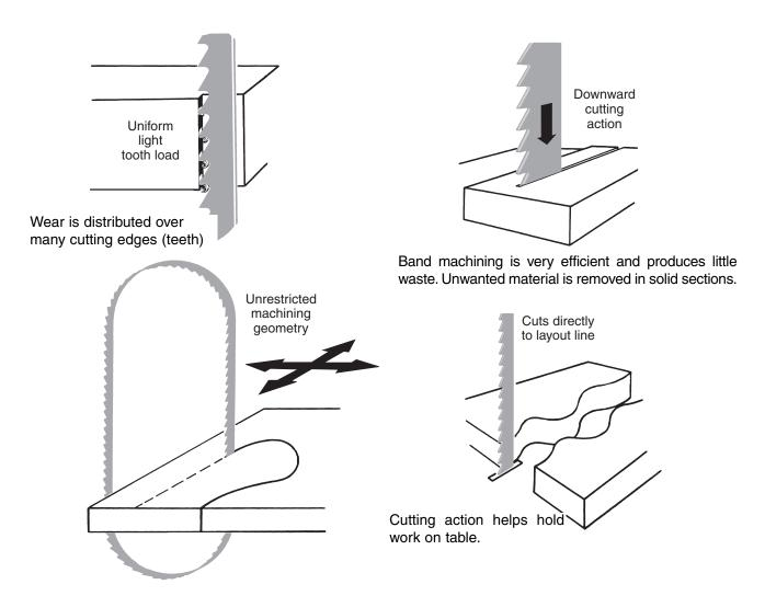
Band machining permits machining at any angle or direction. Cut length is almost unlimited.
