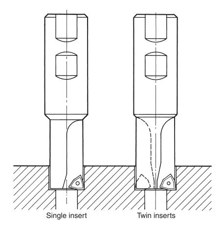
Counterbores with carbide indexable inserts. The inserts are rotated when a cutting edge becomes dull.
