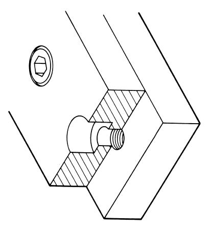
A sectional view of a hole that has been drilled and counterbored to receive a socket-head screw.
