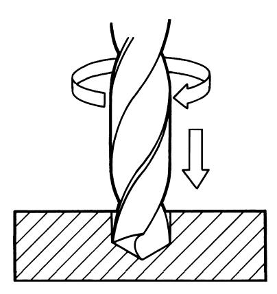
Drilling is the operation most often performed on a drill press. Both rotating force and a downward pushing force are needed for drilling.
