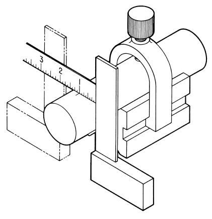
To align the hole for drilling through exact center, place the work and Vblock on the drill press table or on a surface plate. Rotate the punch mark until it is upright. Place a steel square on the flat surface with the blade against the round stock as shown above. Measure from the square blade to the punch mark, and rotate the stock until the measurement is the same when taken from both sides of the stock.
